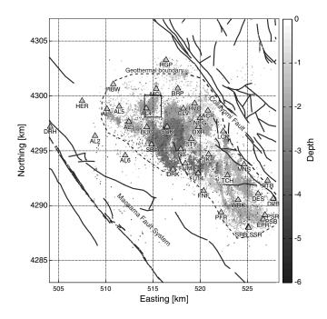
▲ Figure 7. Map view of The Geysers geothermal field with the seismic activity recorded between 2007 and 2012 with  $M_D > 1.0$ . The Lawrence Berkeley National Laboratory (LBNL) seismic network is shown with triangles. The studied area is marked with a black rectangle.
