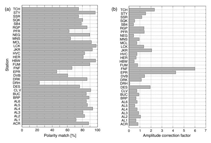
▲ Figure 9. (a) Percentage of polarity matching between observed and theoretical amplitudes at each seismic station of the network in The Geysers geothermal field, determined from the output of the HMT inversion. (b) Amplitude correction factor for each sensor estimated from the HMT inversion.
