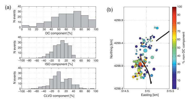
▲ Figure 10. (a) The DC, ISO, and CLVD percentages of the MT solutions derived with the HMT technique. (b) Map view of the induced seismic events with and trajectories of nearby injection wells (black lines). The open-hole section of Prati-9 is indicated by the orange line. Color is encoded with the non-DC percentage of the MT solution, and circle size scales with the earthquake magnitude.
