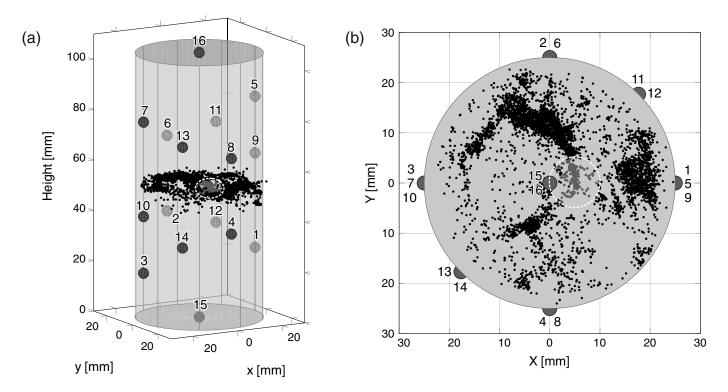
▲ Figure 5. Sensor network geometry and acoustic emission (AE, black dots) activity during the laboratory experiment. AE sensors are glued directly on the deformed rock specimen. (a) Perspective view and (b) top view. The AE activity in this experiment occurred within a narrow height interval 48–58 m. The AEs selected for the HMT refinement of the calculated MTs are surrounded with a dashed ellipses.
