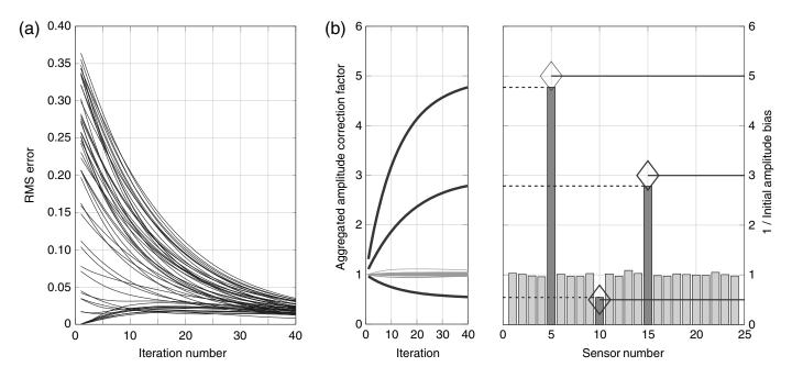
▲ Figure 4. (a) Changes in rms errors of MT solutions with iteration number of the HMT method. (b) Comparison of final amplitude correction factors for all sensors (bars on the right plot) and initial amplitude bias applied to three selected sensors (S5, S10, S15) (rhombs, see Fig. 1 for details).
