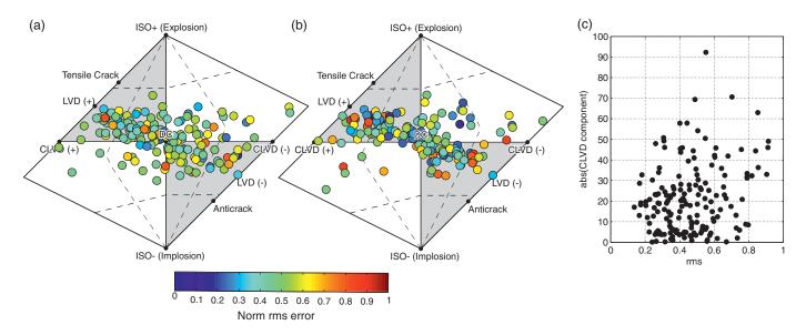
▲ Figure 8. Hudson plots for the 166 estimated MTs of induced seismic events at The Geysers geothermal field, determined by (a) MT inversion using *focimt*, (b) HMT refinement of the original catalog with rms error of MT solution color-encoded, (c) rms error plotted with the absolute value of the CLVD component of the MTs.
